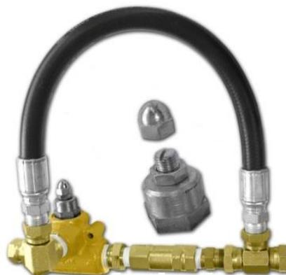
Remove acorn nut, loosen lock nut and turn adjustment screw counter-clockwise to increase speed of the pushgate.
