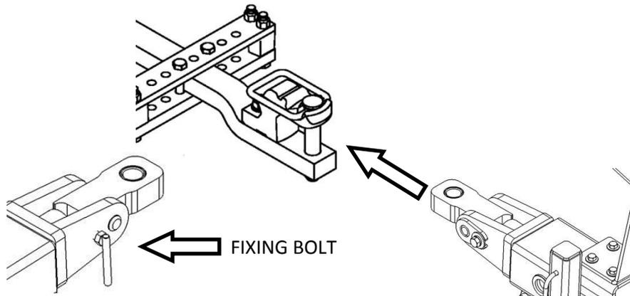
Keep the pull block on horizontal position tightening the fixing bolt. Be sure to loosen the bolt before operating.
